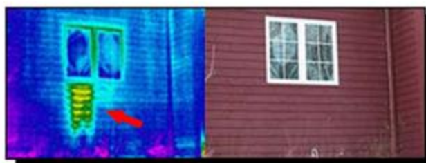
Sunny South's infrared thermal camera can detect insulation flaws as shown above.
